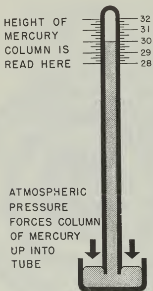
Figure 9-8.—A mercurial barometer.
